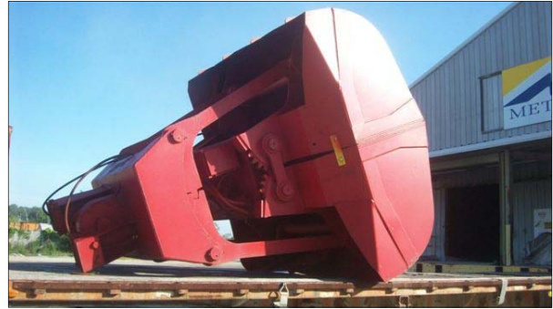
Above is one of the new 14 cubic yard radio controlled grabs and to the left the Mettler Toledo 7260 rail scale that enables us to provide our customers with certified rail weights
